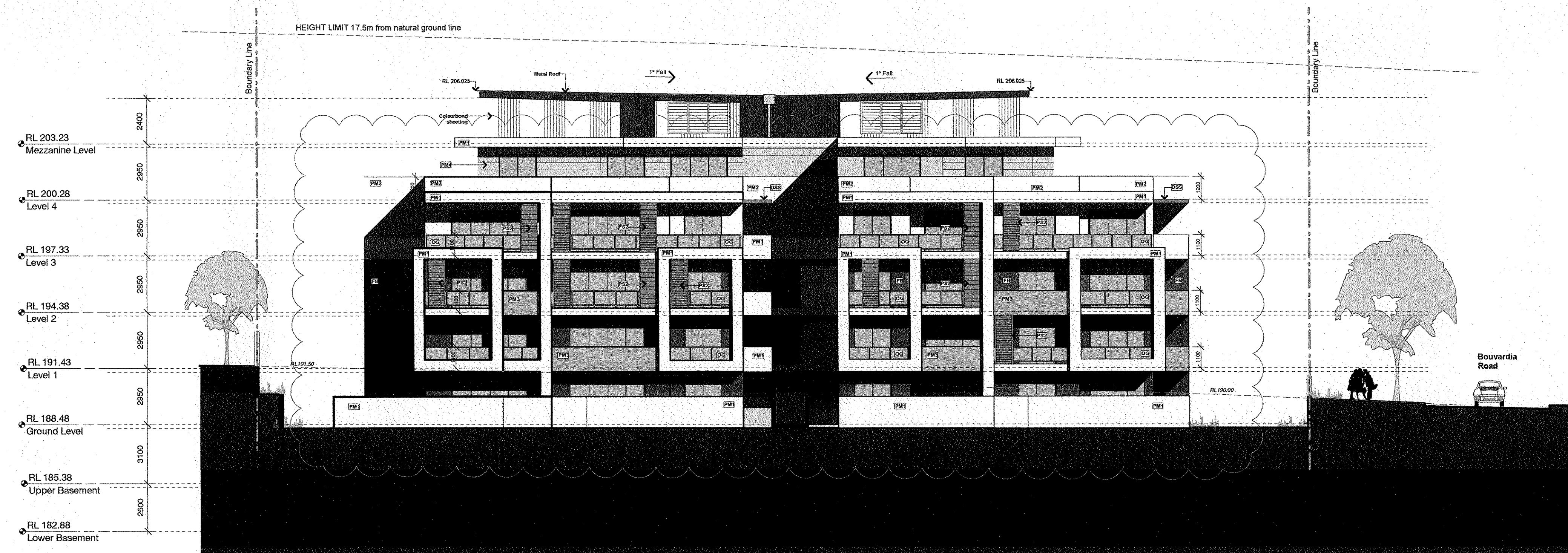
2 South Elevation (Peats Ferry Road) 1:150 @ A1
